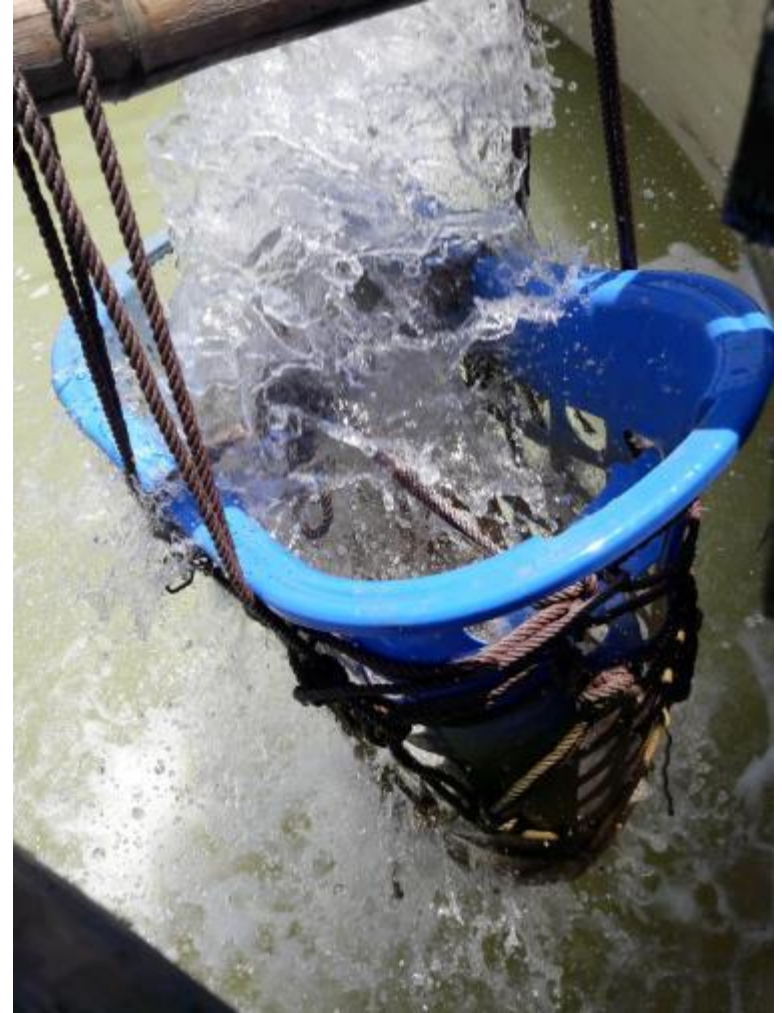
Coagulation with rock alum
